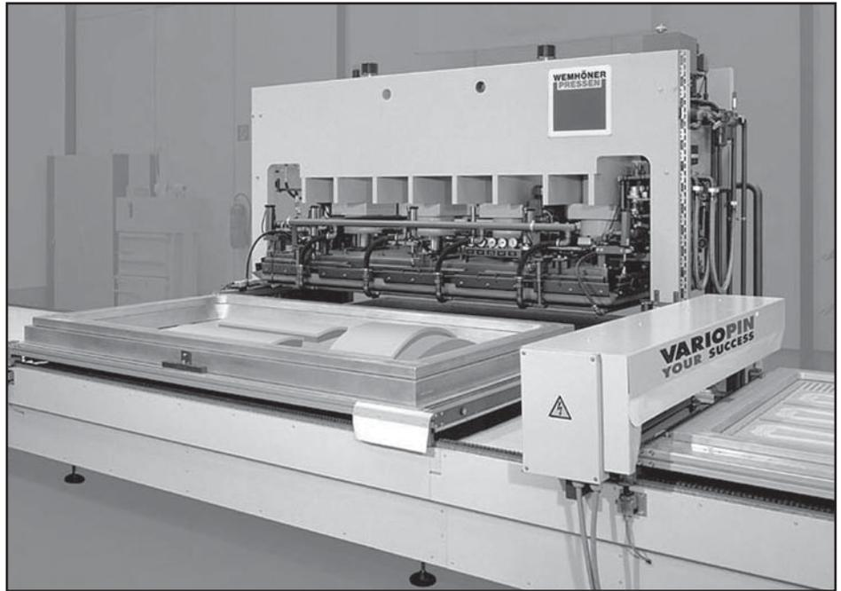
The Wemhöner membrane press is used to make cabinet doors.
