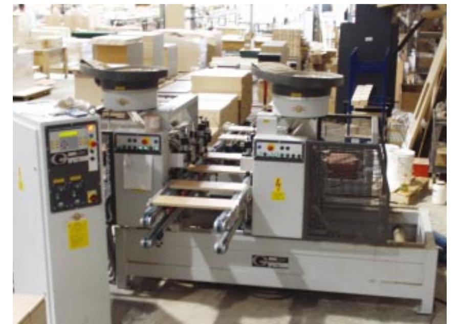
Horizontal drilling and dowel inserting is performed on one of two Gannomat machines. Used for high-production runs, the Spectrum performs double-sided drilling and inserting on more than 2,000 parts per day.
