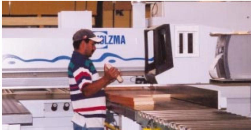
Premier EuroCase has three Holzma programmable panel saws. As parts are cut on the HPP 11, a printed bar code label, which also describes the part in writing, is generated. Roller conveyors and transfer carts are used to transfer the cut parts to the CNC router or boring machines.
