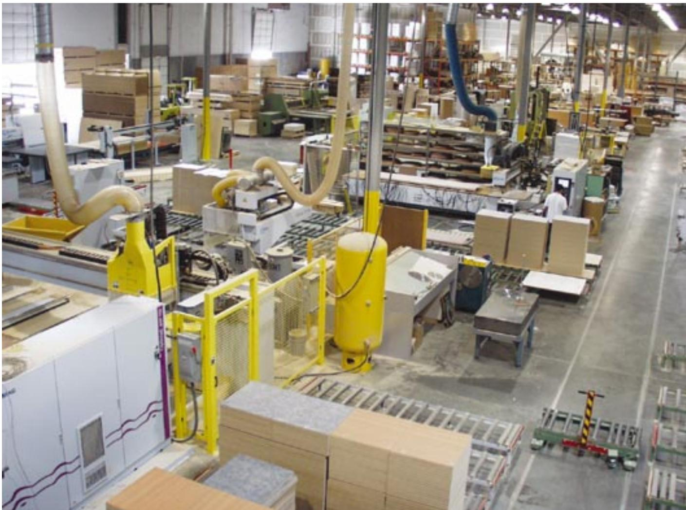
Premier EuroCase’s 70,000-square-foot facility houses more than 20 CNC machines and auxiliary equipment for production manufacturing of store fixtures and laminated components. Programs are downloaded from the office and accessible to all the machines.
