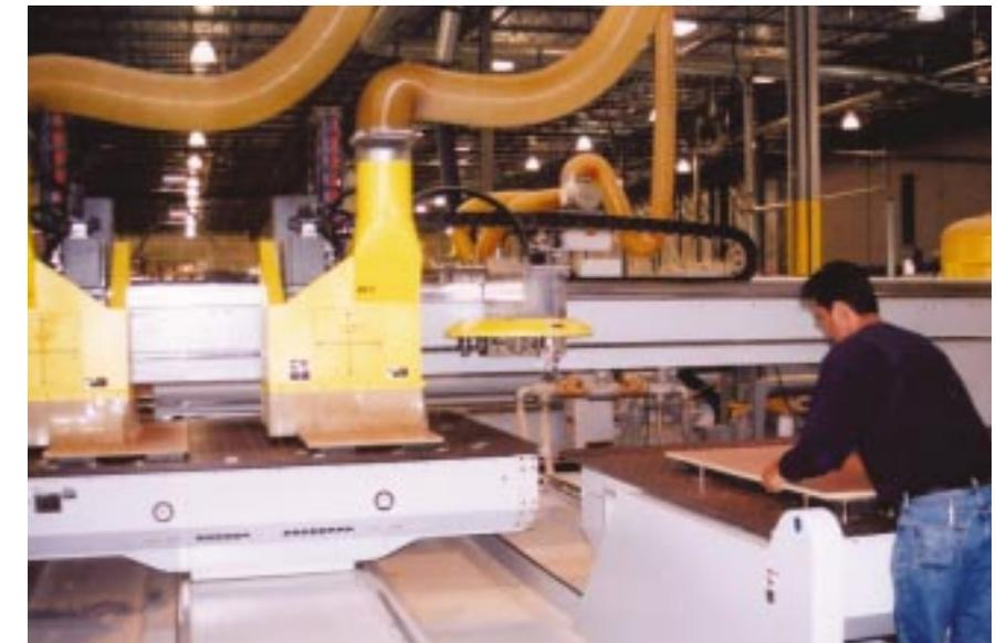
Premier EuroCase’s production rate has increased since acquiring the Homag BOF CNC router. The BOF has Intelligent Processes Optimization technology, allowing the twin-table, twin-head machine to operate in either synchronous-parallel processing or simultaneous independent processing modes. The router spindles can work in tandem or independent of each other, and feature 12-tool ATC units and 12-spindle drilling units.
