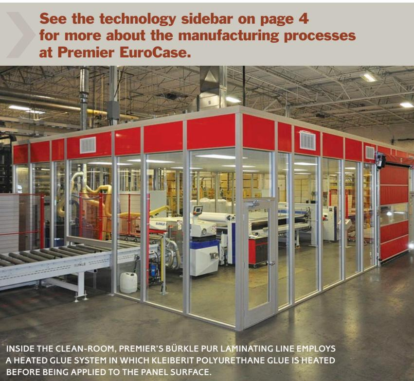
INSIDE THE CLEAN-ROOM, PREMIER'S BÜRKLE PUR LAMINATING LINE EMPLOYS A HEATED GLUE SYSTEM IN WHICH KLEIBERIT POLYURETHANE GLUE IS HEATED BEFORE BEING APPLIED TO THE PANEL SURFACE.
