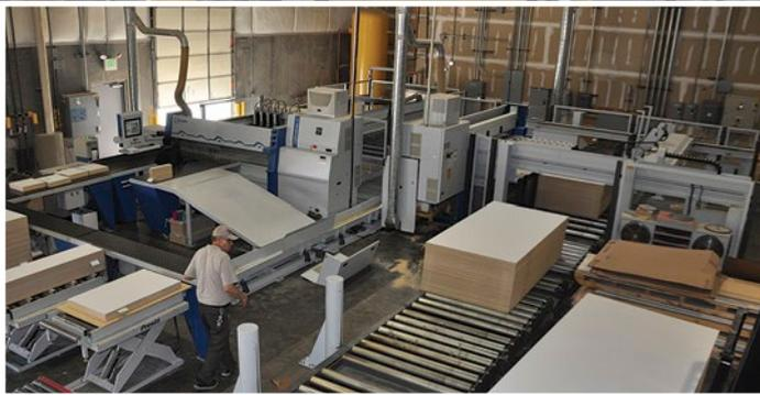
PREMIER'S SIGNIFICANT INVESTMENT IN EQUIPMENT INCLUDES A WEMHONER SHORT-CYCLE MELAMINE PRESS, HOMAG LASER AND TRADITIONAL EDGE BANDERS, HOLZMA PANEL SAWS, AND WEEKE POINT-TO-POINT MACHINES, ALL OF WHICH ARE COORDINATED, NETWORKED AND WORK TOGETHER AS A SYSTEM. THE PREMIER FACILITY ALSO HAS AS A GLASS-WALLED CLASS-100 (ISO5) CLEANROOM AND A BÜRKLE PUR LAMINATING LINE.
